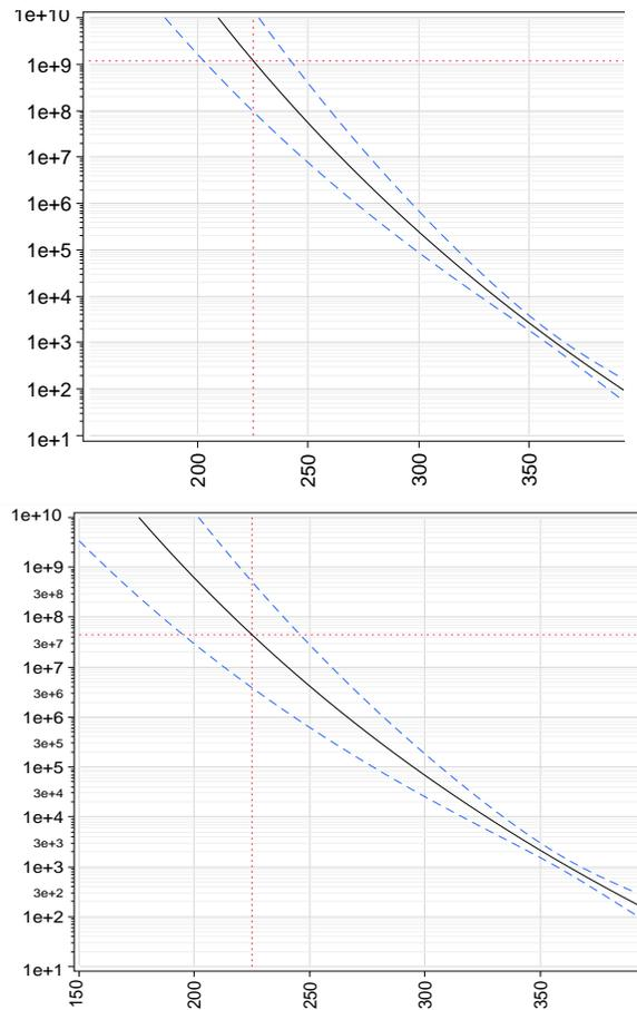
Fig. 2. DC-ALT intrinsic lifetime prediction of G28V3 (upper) and G28V4 (lower) technologies. Solid line shows the time (hours) to 1%-ile failures, and dashed lines show 80% 2-sided (90% 1-sided) statistical confidence bounds, versus junction temperature.
