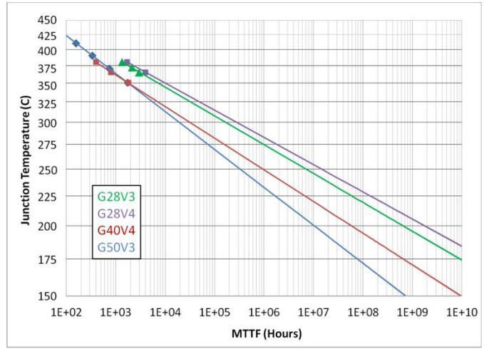
Fig. 7. Median time to failure and intrinsic lifetime extrapolations for G28V3, G28V4, and G40V4 DC-ALT, and G50V3 RF-ALT.
