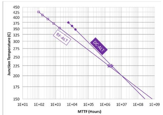
Fig. 5. Median time to failure versus junction temperature for G50V3 RF-ALT and DC-ALT. Stars represent fiducial points to illustrate the predicted lifetime at maximum rated junction temperature of 225 °C.
