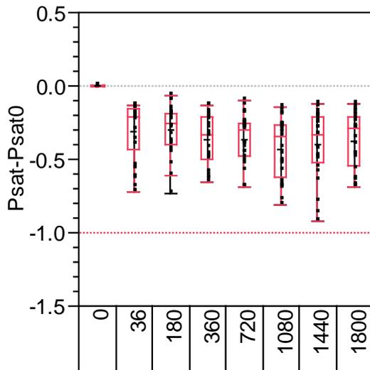
Fig. 3. Representative PSAT degradation (dB) versus hours for G50V3 technology DC-ALT at a typical accelerated stress junction temperature. Each data point represents one device under test at its corresponding down point duration. The red line indicates the failure criterion of -1 dB.
