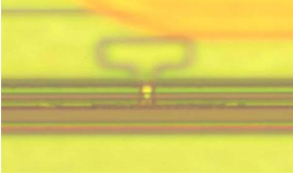
Fig. 6. Representative visual inspection image showing field plate voiding after a duration of RF-ALT stress, but prior to catastrophic failure.
