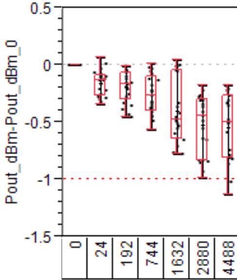
Fig. 1. Representative saturated output power degradation (dB) versus hours for G28V3 technology DC-ALT at a typical accelerated stress junction temperature. Each data point represents one device under test at its corresponding down point duration. The red line indicates the failure criterion of -1 dB.
