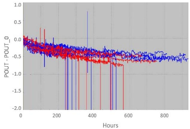
Fig. 4. Representative POUT degradation (dB) versus hours for a set of G50V3 devices under RF-ALT at a typical accelerated stress junction temperature. The red and blue curves represent sets of devices that can be considered equivalent for the purposes of this test.
