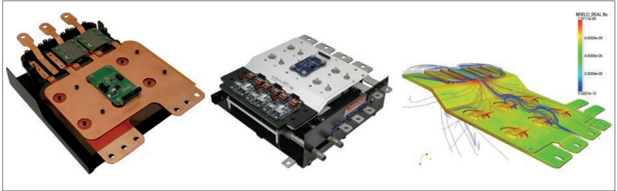
Figure 2: An initial bussing design V1 (left), and optimized design V2 (middle), for a 3-phase inverter using the Wolfspeed CAS325M12HM2 power module. The magnetic flux B_x for the low-inductance ( \sim 3.5 nH) V2 bussing is shown (right)
