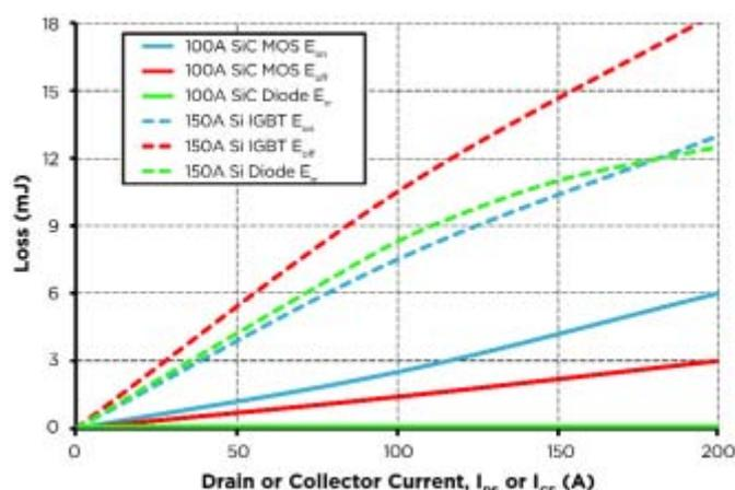
Figure 2b: switching loss (switch and diode) for 150A Si IGBT and 100A SiC MOSFET at 150°C
