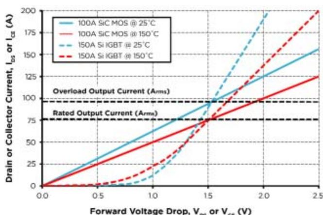
Figure 2a: Conduction loss for 150A Si IGBT and 100A SiC MOSFET at 25°C and 150°C
