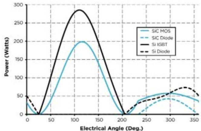
Figure 3: Total loss (switch and diode) of the 100A SiC MOSFET and the 150A Si IGBT modules for the 75A<sub>rms</sub> and 5kHz condition.
