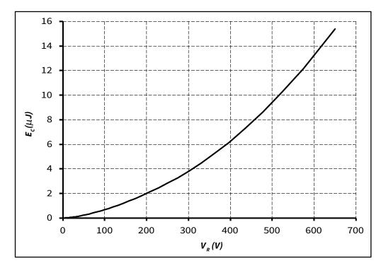
Figure 7. Typical Capacitance Stored Energy
