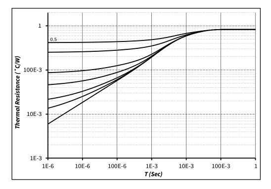
Figure 8. Transient Thermal Impedance
