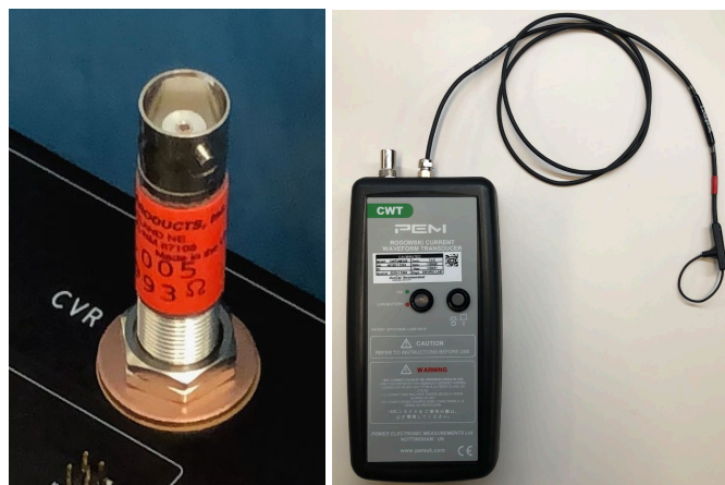
Figure 8. Probe examples, (a) current viewing resistor (T & M Research SSDN-005, 400 MHz), (b) Rogowski current probe (PEM CWTUM/3/B, 30 MHz)
