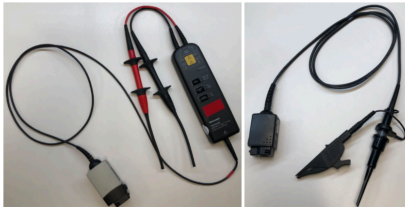
Figure 12. Probe examples, (a) Tektronix differential probe THDP0200 (1500 V Range), (b) Tektronix TPP0850 voltage probe
