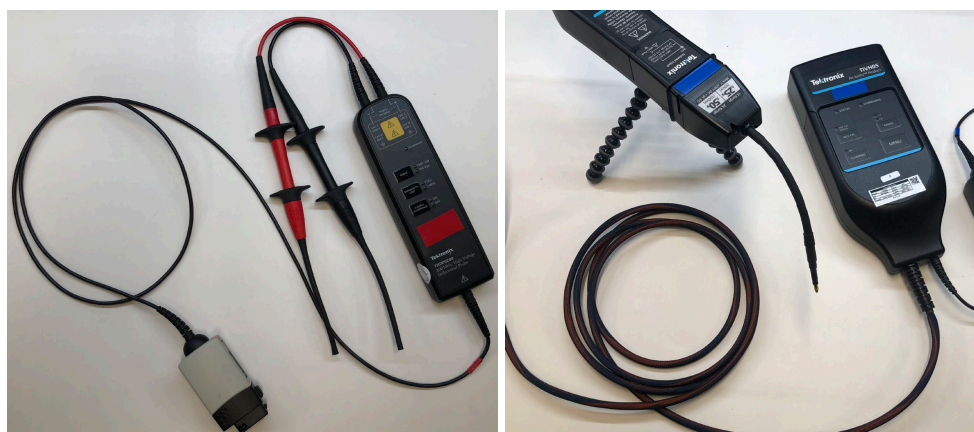
Figure 14. Probe examples, (a) Tektronix differential probe THDP0200 (150 V Range), (b) Tektronix IsoVu TIVH05 (TIVPMX10X, ±25 V sensor tip)
