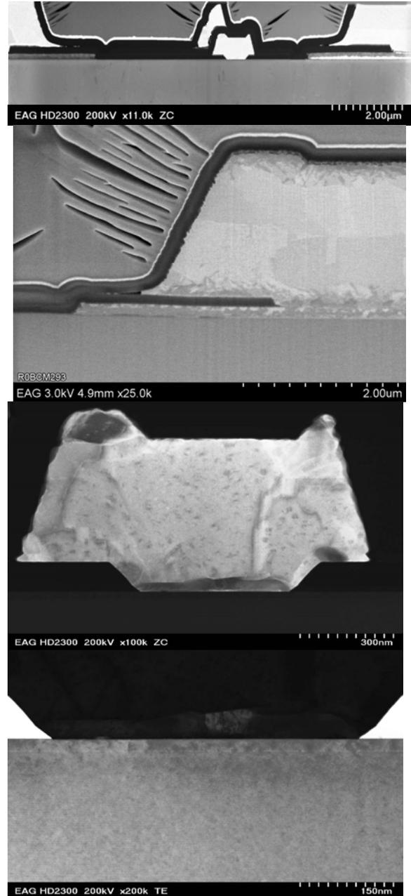
Fig. 4. Electron microscope images of a HEMT device after ALT stress that induced 1 dB degradation in saturated power.
