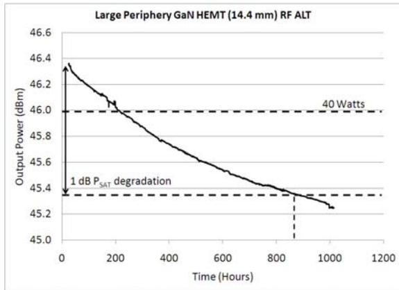
Fig. 5. Output power versus time for a large periphery (14.4 mm) GaN HEMT device under RF ALT stress conditions of 28 V,  $I_{dq} = 1.0$  A, input power 37 dBm, dissipated power 3.3 W/mm, case temperature of 200 °C and junction temperature of 380 °C.
