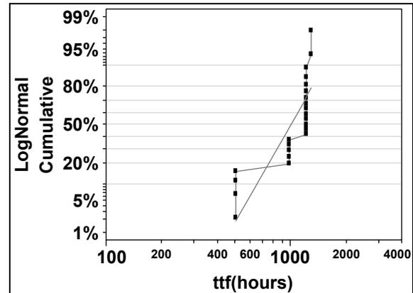
Fig. 3. Lognormal lifetime distribution for 24 devices fabricated on 100 mm wafers at ALT conditions at 380 °C junction temperature.
