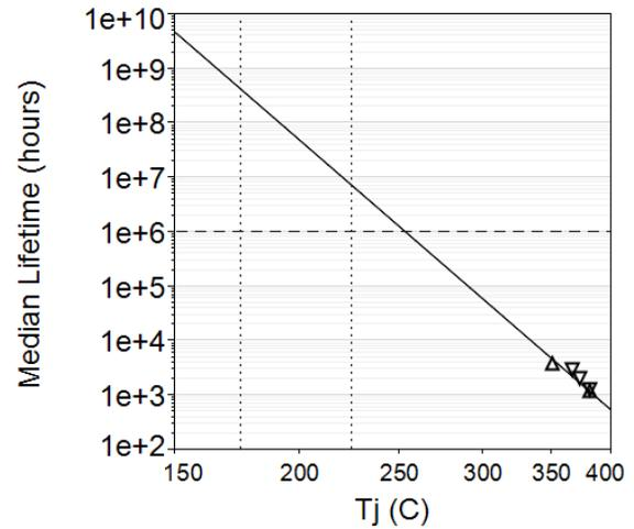
Fig. 2. Median lifetime versus junction temperature for 28 V DC ALT at 6 W/mm on devices fabricated on 100 mm (triangles) and 3'' (inverted triangles) SiC wafers. Solid line is Arrhenius fit to all data and extrapolation to operating conditions.
