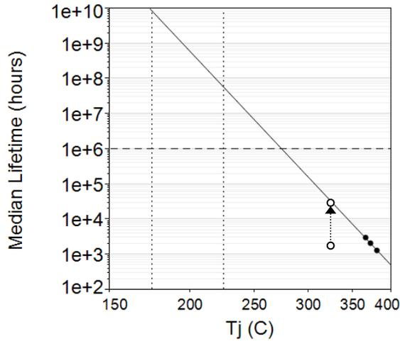
Fig. 1. Median lifetime versus junction temperature for 28 V DC ALT at 6 W/mm on devices fabricated on 3'' SiC wafers. Solid symbols represent median lifetimes of 10-15 devices per stress temperature. Open symbols represent a suspended test with lifetime extrapolated to 1 dB saturated power degradation. Solid line is Arrhenius fit to solid symbols and extrapolation to operating conditions.
