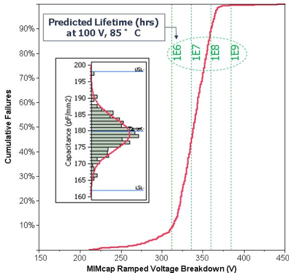
Fig. 6. MIM capacitor ramped voltage breakdown distribution. Dashed lines show predicted lifetime at 100 V and 85 °C. Inset
