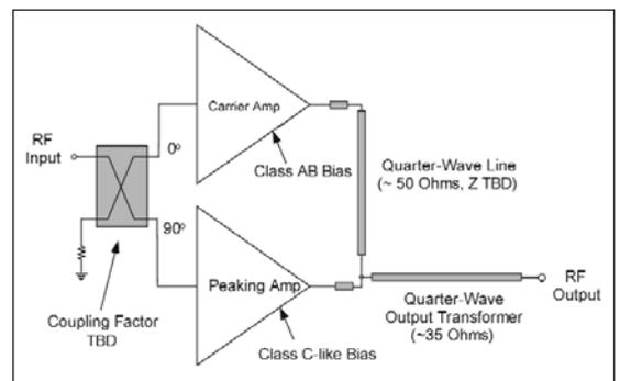
Figure 1 · A basic 2-way Doherty amplifier configuration.
