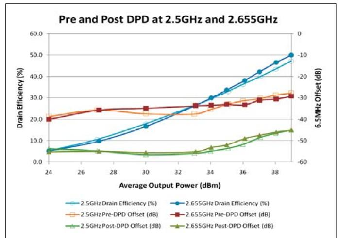
Figure 16 · Doherty amplifier spectral mask vs. average output power, with and without DPD correction (F = 2.5, 2.655 GHz,  $V_{supply} = +28$  V).
