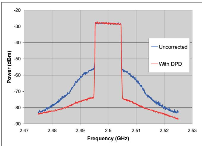
Figure 15 · Doherty amplifier spectral mask, with and without DPD correction (F = 2.5 GHz,  $P_{ave} = 8$  watts,  $V_{supply} = +28$  V,  $I = 600$  mA, 48% DC-RF efficiency).
