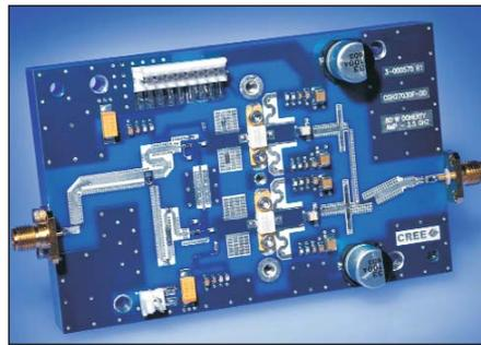
Figure 8 · The 2.5-2.7 GHz Doherty amplifier with two 30W GaN HEMTs PCB size is 2.5 × 4.0 inches.
