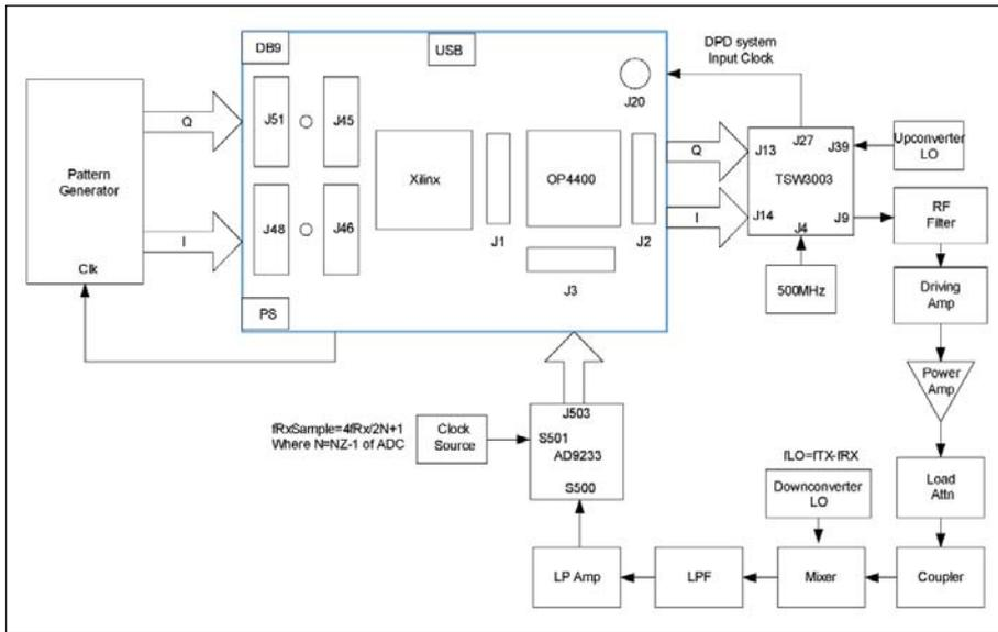
Figure 14 · Digital predistortion test-bed using Optichron OP4400 chipset.
