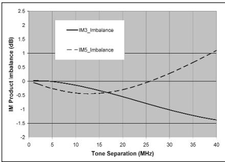
Figure 7 · Simulated 2-tone IM products imbalance versus frequency separation of tones ( $P_{out} = +32$  dBm).
