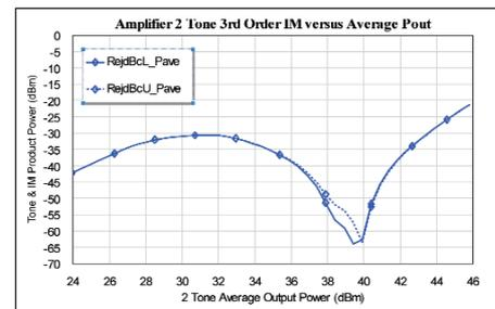
Figure 6 · Simulated 2-tone intermodulation products versus output power level (tone separation of 1 MHz).
