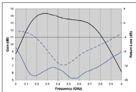
Figure 11 · Measured small-signal gain and input and output return loss versus frequency (output return loss is dashed line).
