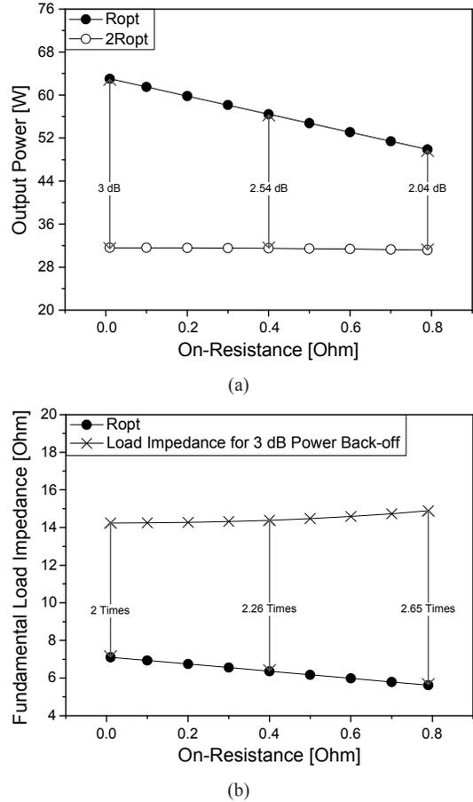
Fig. 3. (a) Maximum output powers employing  $R_{opt}$  and  $2R_{opt}$  with varying  $R_{on}$  from 0 to 0.8  $\Omega$ . (b)  $R_{opt}$  and load impedance for 3 dB power back-off with varying  $R_{on}$  from 0 to 0.8  $\Omega$ .
