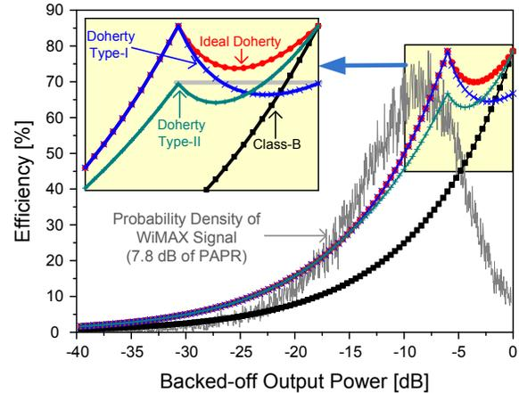
Fig. 1. Ideal efficiencies of the class-B and two-way Doherty power amplifiers and the probability density of a WiMAX signal with a 7.8 dB PAPR.
