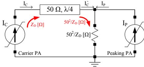
Fig. 5. Operational diagram of the proposed Doherty amplifier.
