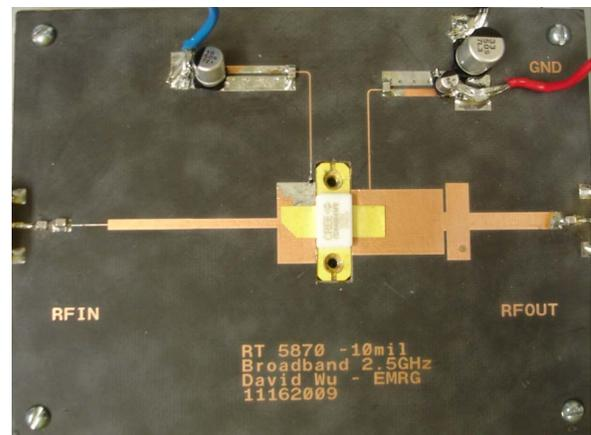
Fig. 6. Fabricated input and output matching network
