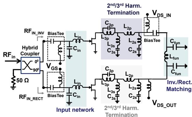
Fig. 1. Simplified schematic of the UHF class E<sup>2</sup> converter.
