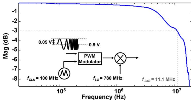
Fig. 5. Measured small-signal versus frequency response. Details of the implemented PWM for this experiment appear in the inset.
