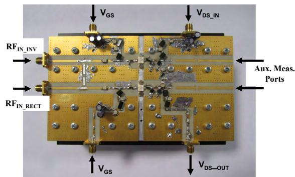
Fig. 2. Photograph and details of the implemented converter.
