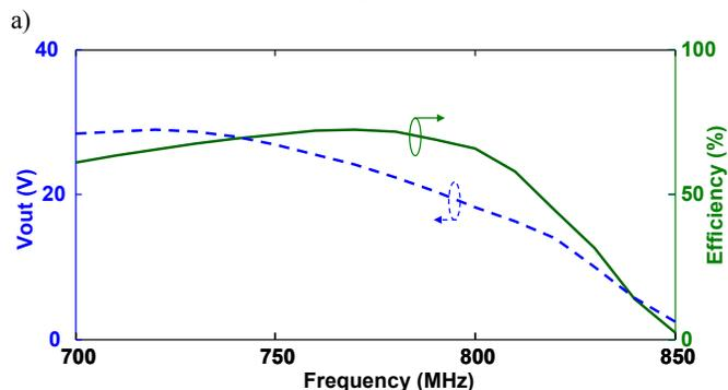
Fig. 3. (--) Output voltage and (—) efficiency versus a) input voltage ( $f = 780$  MHz) and b) switching frequency ( $V_{DD} = 28$  V).
