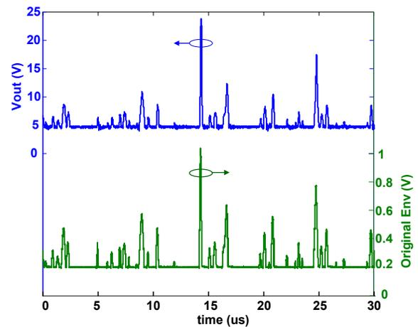
Fig. 6. (–) Original and (–) recovered clipped WCDMA envelope signals, as used in ET or hybrid ET/EET wireless transmitters.
