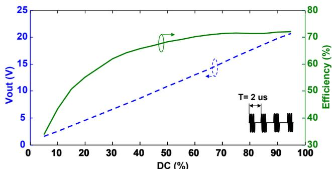
Fig. 4. (--) Measured output voltage and (—) efficiency profiles versus envelope duty cycle at  $V_{DD} = 28$  V and  $f = 780$  MHz.
