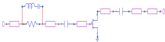
Figure 2. Simplified CGH55015-TB and CGH55030-TB amplifier topologies
