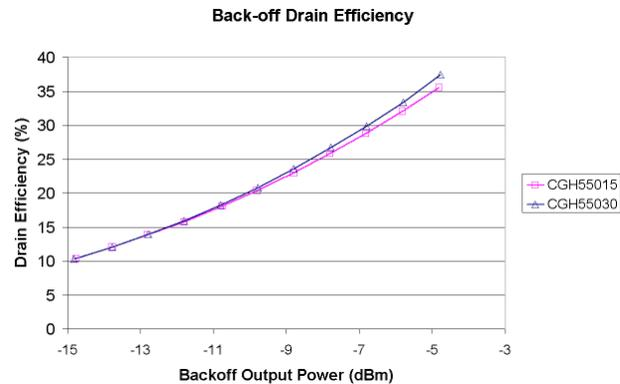
Figure 9. Measured drain efficiency vs. back-off for the CGH55015-TB and CGH55030-TB amplifier circuits
