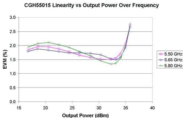
Figure 10. Measured EVM vs. average output power for the CGH55015-TB reference amplifier across frequency
