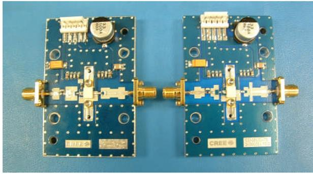
Figure 6. Photograph of CGH55015-TB and CGH55030-TB amplifier circuits with GaN HEMT devices
