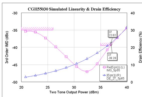
Figure 5. Simulation of linearity and efficiency vs. two tone output power for the CGH55030-TB amplifier @ 5.65 GHz
