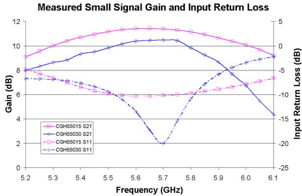
Figure 7. Measured small signal performance of the CGH55015-TB and CGH55030-TB amplifier circuits with GaN HEMT devices
