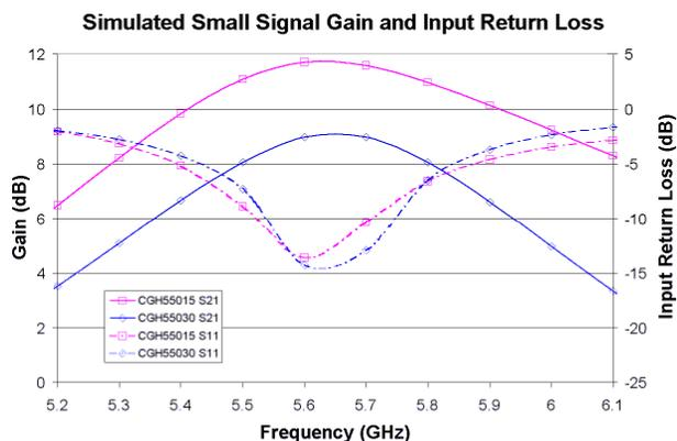
Figure 3. CGH55015-TB and CGH55030-TB amplifier small signal simulation
