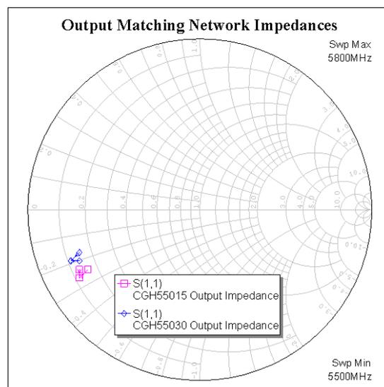
Figure 1. CGH55015 and CGH55030 transistor output impedances
