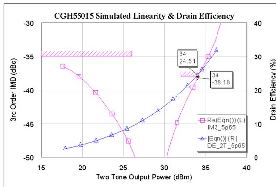
Figure 4. Simulation of linearity and efficiency vs. two tone output power for the CGH55015-TB amplifier @ 5.65 GHz
