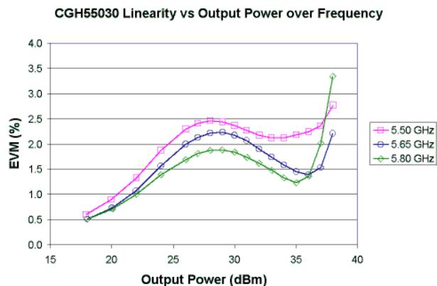
Figure 11. Measured EVM vs. average output power for the CGH55030-TB reference amplifier across frequency
