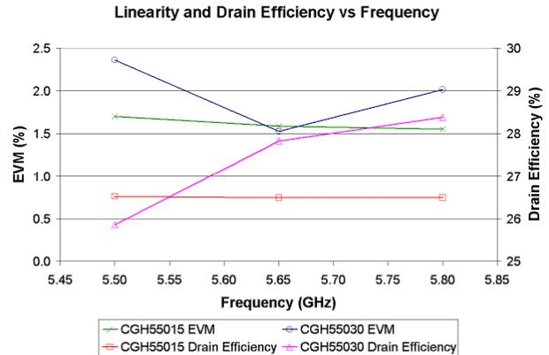
Figure 8. Measured EVM and efficiency vs. frequency of the CGH55015-TB and CGH55030-TB reference amplifiers
