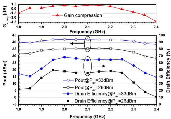
Fig. 6. CW measured performances versus frequency at 33 dBm of input power.
