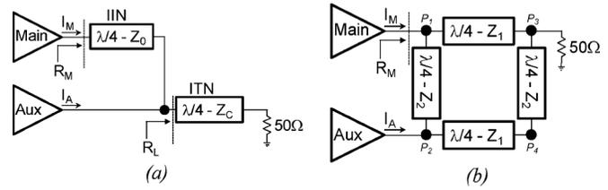
Fig. 1. (a) Typical and (b) proposed DPA implementation.
