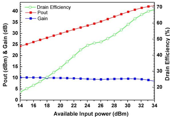
Fig. 5. CW measured performances versus input power at 2 GHz.
