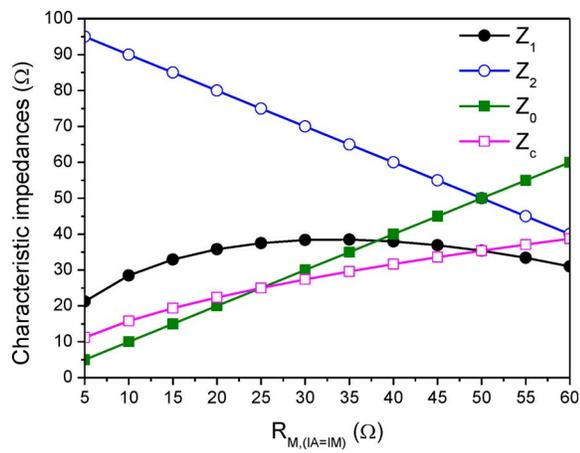
Fig. 2. Behaviors of the characteristic impedances of the  $\lambda/4$ -TLines in the proposed combiner and in the standard approach.
