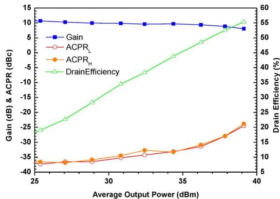
Fig. 7. WiMAX measured performances at 2.1 GHz.
