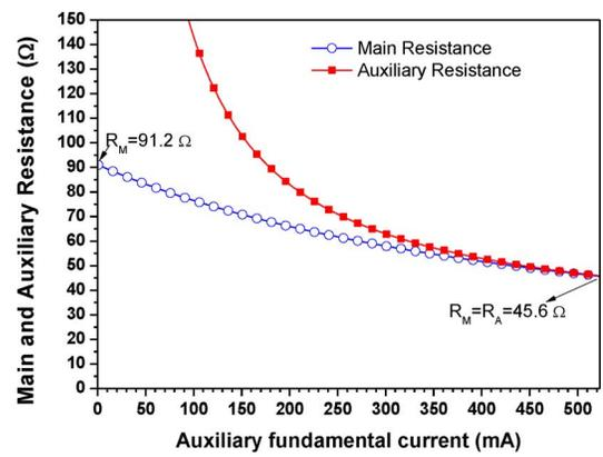
Fig. 3. Devices' loads as a function of the Auxiliary current.
