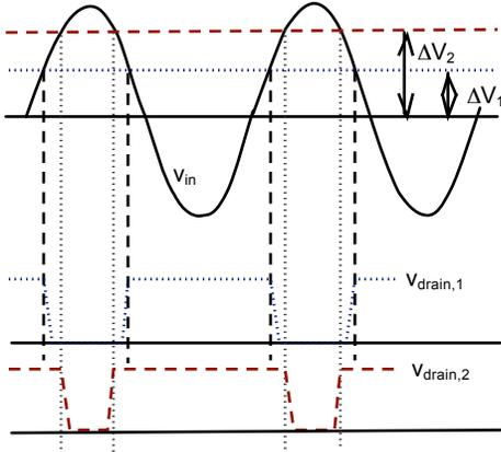
Fig. 2. Operating principle of the power amplifier. The difference  $\Delta v$  between  $V_{bias}$  and  $V_{th}$  varies, depending on  $V_{bias}$ , and the resulting pulse width modulated drain voltage is illustrated for two cases.
