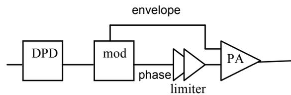
Fig. 1. Transmitter architecture.
