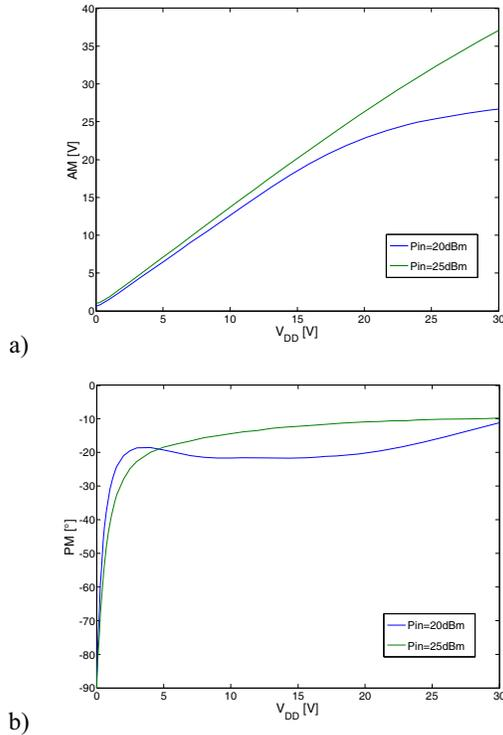
Fig.2. a) V<sub>dd</sub>-to-AM and b) V<sub>dd</sub>-to-PM static characteristics.
