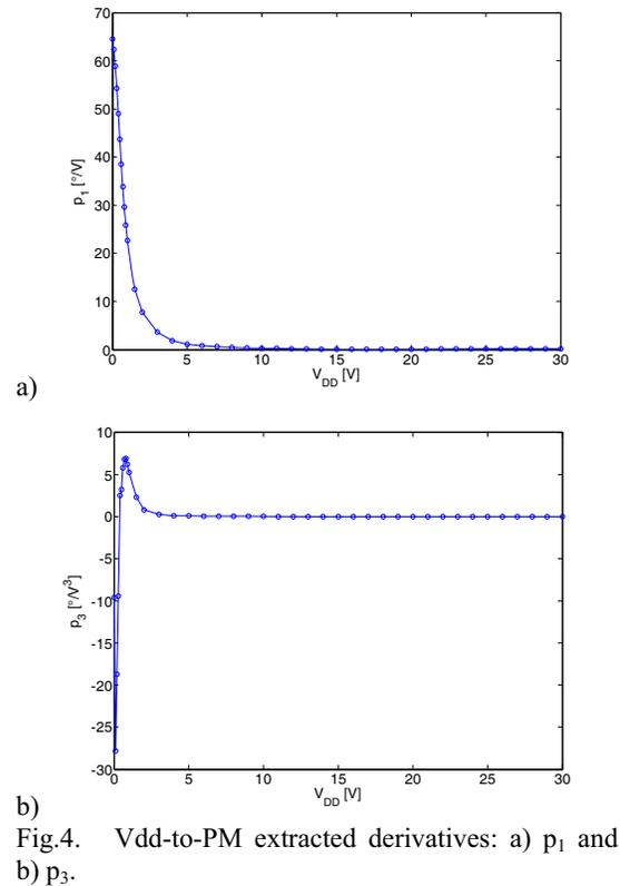
Recently, a comprehensive study was employed to accurately describe the Vdd-to-AM and Vdd-to-PM profiles of a PHEMT based class E PA [5]. The nonlinear gate-to-drain capacitance in the device equivalent circuit was shown to be responsible for the observed behavior.
