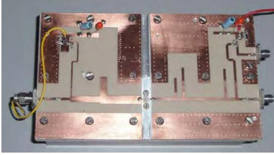
Fig.1. Image of the implemented class E PA.
