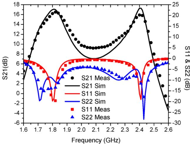
Figure 4. Measured and simulated S-parameters of the dual-band PA.
