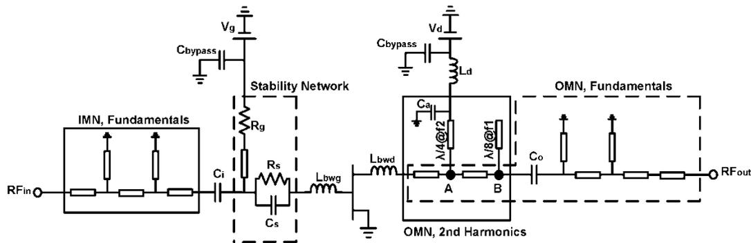
Figure 2. Circuit diagram of the dual-band PA.
