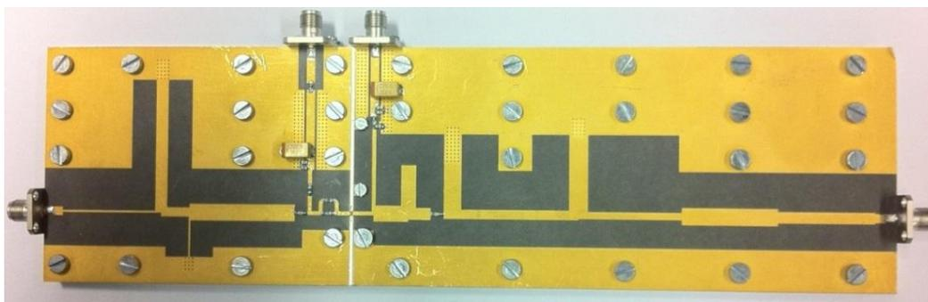
Figure 3. Photo of the implemented dual-band PA, size =  $6 \times 20$  cm<sup>2</sup>.
