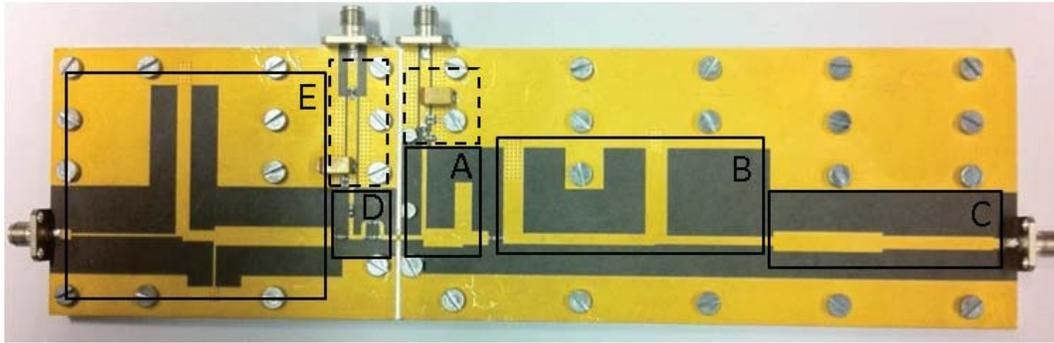
Fig. 1. Photos of the realized dual-band PA. Box 'A' is the network for the 2nd harmonics control. Box 'B' is the network for the synthesis of the reactive part of the loads at fundamentals. Box 'C' is the network for the transformation from the 50 Ohm termination to the optimum output resistance at the fundamentals. Box 'D' is the stabilization network. Box 'E' is the input matching network. Dashed boxed are the DC filtering networks.
