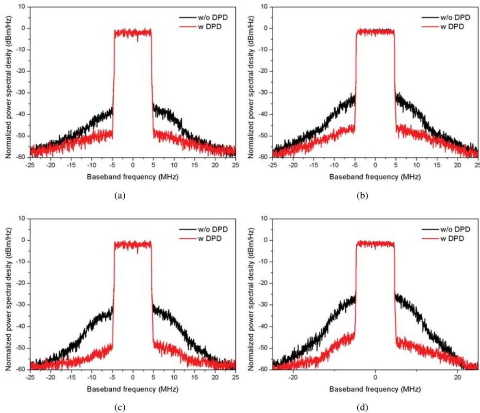
Fig. 4. Output signal spectrum, without (w/o) and with (w) DPD, of (a) dual-band PA by using a 10MHz LTE signal at center frequency of 1.8GHz, (b) dual-band PA by using a 10MHz WiMAX signal at center frequency of 2.4GHz, (c) dual-band DPA by using a 10MHz LTE signal at center frequency of 1.8GHz and (d) dual-band DPA by using a 10MHz WiMAX signal at center frequency of 2.4GHz. Both PA and DPA have been tested in concurrent mode.
