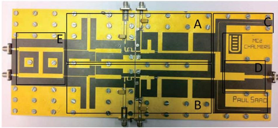
Fig. 2. Photos of the realized dual-band DPA. Box 'A' is the dual-band Main amplifier. Box 'B' is the dual-band Auxiliary amplifier. Box 'C' is the dual-band  $\lambda/4$ . Box 'D' is the network for the transformation from the 50 Ohm termination to the optimum output resistance. Box 'E' is the wide-band unbalanced input power splitter.
