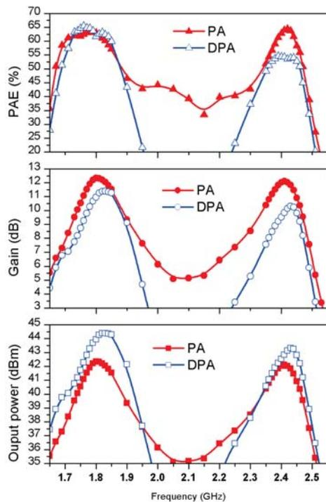
Fig. 3. CW measurements of dual-band PA and dual-band DPA.
