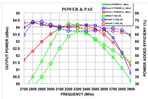
Figure 2. Simulations comparing the relative bandwidth of three different matching topologies
