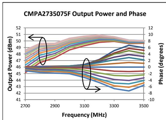
Figure 11. Variation in magnitude and phase due to changes in input power
