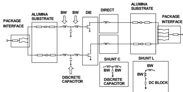
Figure 1. Hybrid transistor output matching topologies
