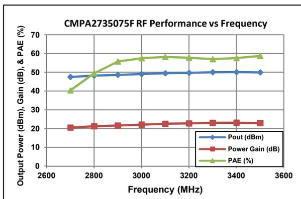
Figure 11. Typical performance of the CMPA2735075F
