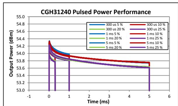
Figure 8. Amplitude droop performance of CGH31240F
