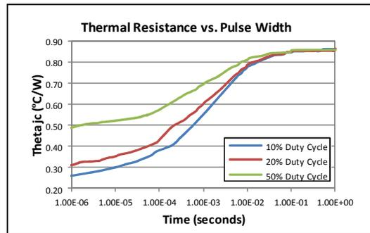
Figure 7. Transient thermal behavior of CGH31240F
