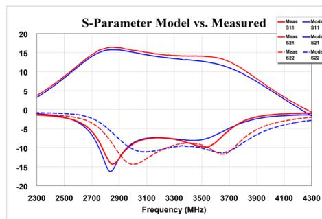
Figure 4. Small signal performance of CGH35240F
