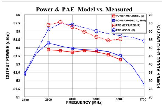
Figure 5. Large Signal performance of CGH35240F
