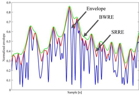
Fig. 4. Time representation of the envelope and its SR and BW limited versions.
