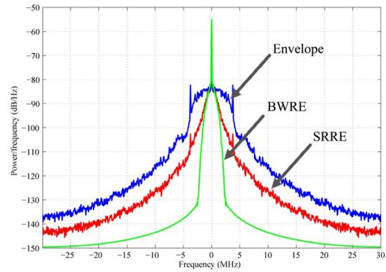
Fig. 5. Frequency representation of the envelope and its SR and BW limited versions.
