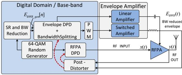
Fig. 2. Block diagram of the proposed ET architecture.
