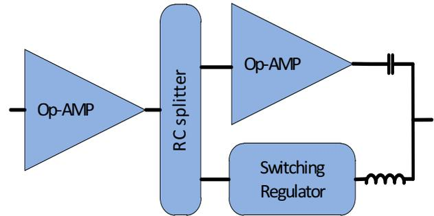
Fig. 1. Hybrid envelope amplifier for EER proposed in [1].
