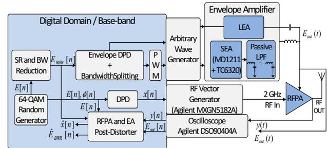
Fig. 6. Block-diagram of the experimental ET set-up.
