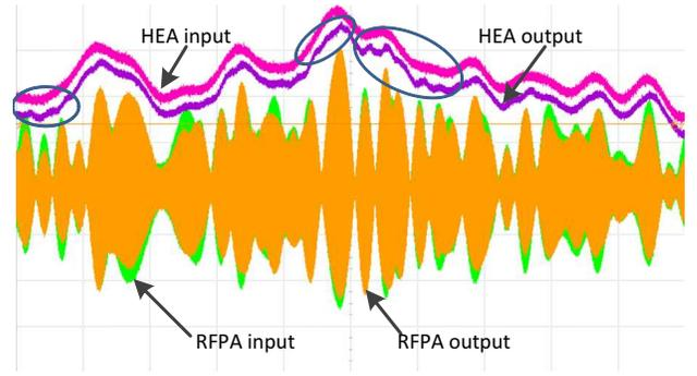
Fig. 3. RFPA and EA inputs and outputs.
