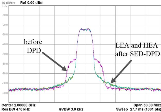
Fig. 8. Spectrum of a 64-QAM signal before and after SED-DPD when the BW reduced envelope is used as dynamic supply.
