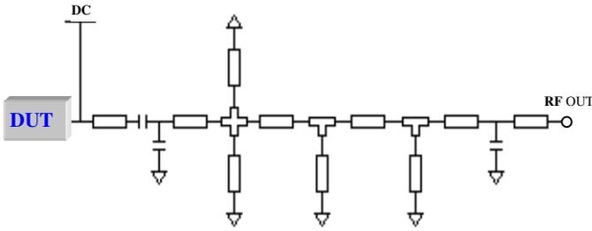
Fig. 3. Continuous class-F output matching network schematic
