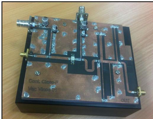
Fig. 7. Realized Continuous Class-F 10W power amplifier.
