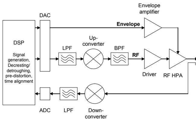
Fig.2: Block diagram of EER/ET amplifier system
