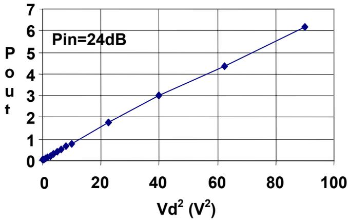
Fig.1: Output power (in W) for CW inputs to Class E amplifier vs square of supply voltage.
