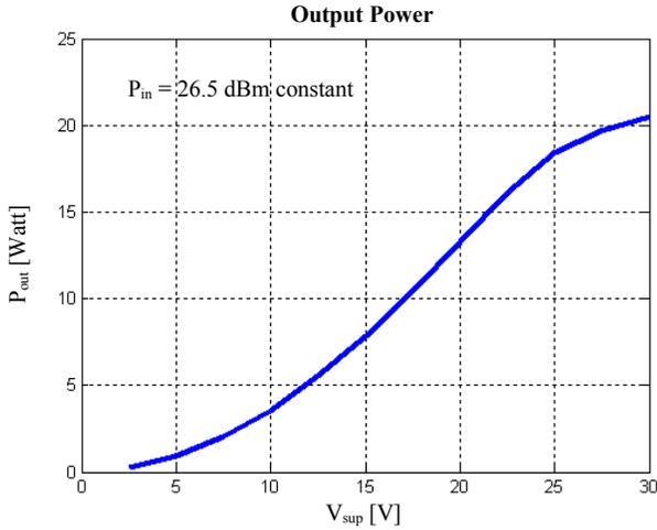
Figure 4. Output power versus drain supply voltage
