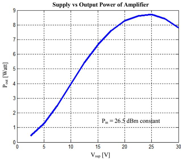
Figure 8. Measured dependency of  $P_{out}$  on the drain supply voltage  $V_{sup}$
