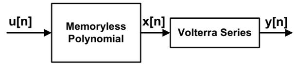
Fig. 4. Block diagram of Enhanced Hammerstein behavior model.
