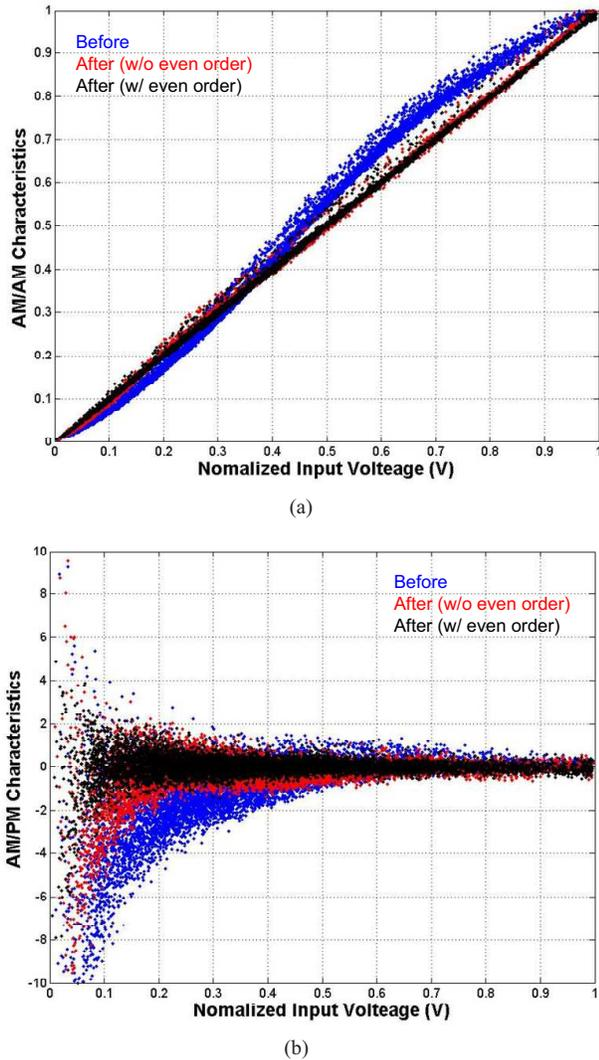
Fig. 7. Measured (a) AM-to-AM and (b) AM-to-PM characteristics.
