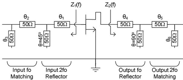
Fig. 4. Topology of the prototype SiC MESFET and GaN HEMT-based frequency doublers.
