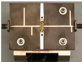
Fig. 5. Photo of GaN HEMT-based frequency doubler.
