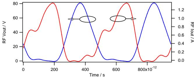
Fig. 6. De-embedded output RF waveforms for  $V_{ds}=28V$ .
