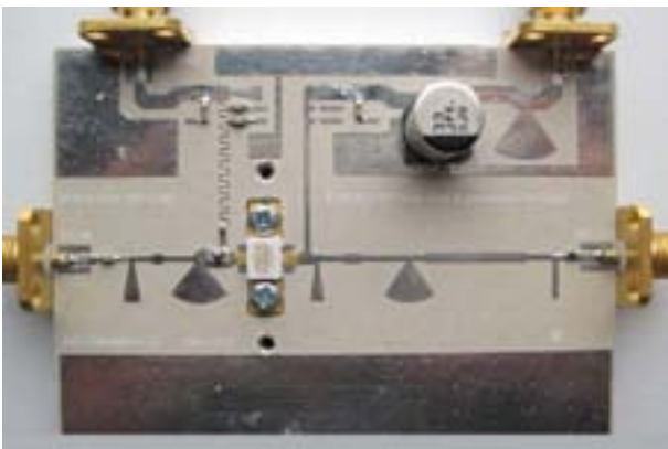
Fig. 8. The fabricated PA mounted on an aluminum heat sink.
