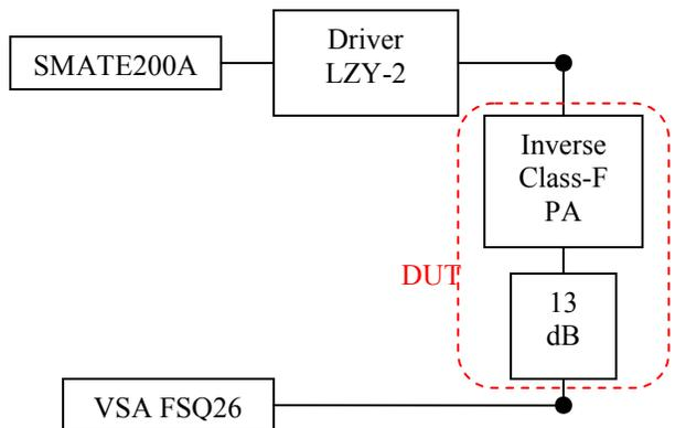
Fig. 1 Measurement setup for AM-AM and AM-PM Characterization
