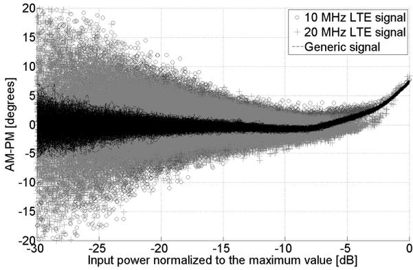
Fig. 5 AM-PM of the PA in presence of the generic signal and some 3GPP LTE signals
