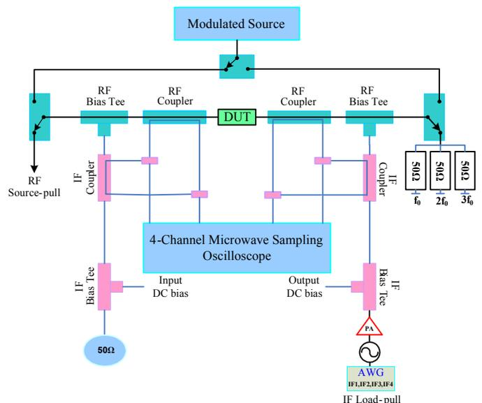
Fig. 1 Modulated waveform measurement system with active baseband load-pull.
