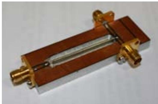
Fig. 3: Simple coaxial cable transmission line balun.
