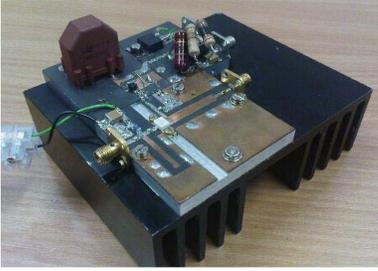
Fig. 2. The implemented Integrated AET Block
