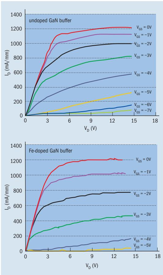
**Fig. 3.** Switching from an undoped to an iron-doped buffer improves the HEMTs' pinch-off characteristics (a smaller gate voltage is required to extinguish the drain current), and consequently increases the device's output power and efficiency.
