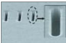
Cree offers both epiwafers and device/MMIC foundry services for Ka- and Q-band applications. Through these services, Cree's customers can gain access to the company's field-plated, electron-beam lithography GaN MMIC technology. An individual source via process (shown above) has recently been applied to SiC substrates, enabling microstrip MMICs delivering even higher total power, gain and efficiency than those of the devices described in this article.
