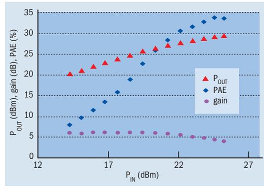
**Fig. 4.** Cree's latest 100  $\mu\text{m}$  wide devices can deliver 8.6 W/mm at 40 GHz with a power-added efficiency (PAE) of 34%. This is a significant improvement over the performance of generic GaN HEMTs produced using electron-beam lithography, which generate 3–4 W/mm at PAEs of 20–30%.
