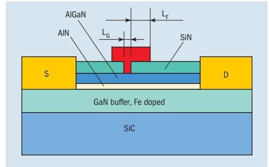
Fig. 1. Cree's GaN HEMTs were grown by MOCVD on a semi-insulating SiC substrate. An AlN nucleation layer was deposited first, followed by a 2–4 μm thick iron-doped GaN buffer, a strained thin AlN layer and a 22 nm thick AlGaN barrier. Ohmic contacts were produced by annealing a Ti/Al/Ni/Au alloy at 880 °C. A Ni/Au contact formed the Schottky gate, after the dimensions were defined by electron-beam lithography and subsequent dry etch through a SiN layer.
