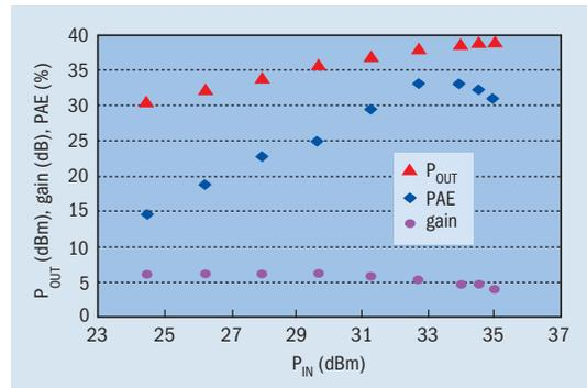
**Fig. 5.** GaN HEMTs can slash the footprint of the power amplifier. This GaN-based pre-matched 1.5 mm wide device generates a record 8.05 W at 30 GHz. To produce the same power with GaAs MMIC requires a device 10 times wider.
