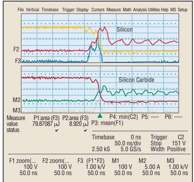
Fig. 7. MOSFET turn-on loss in PFC front-end converter.
