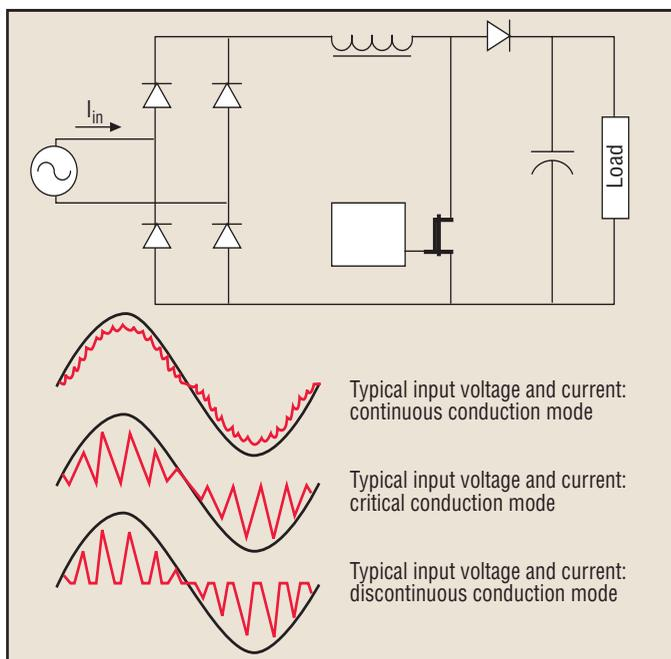
Fig. 1. Comparison of conduction modes for a boost converter.
