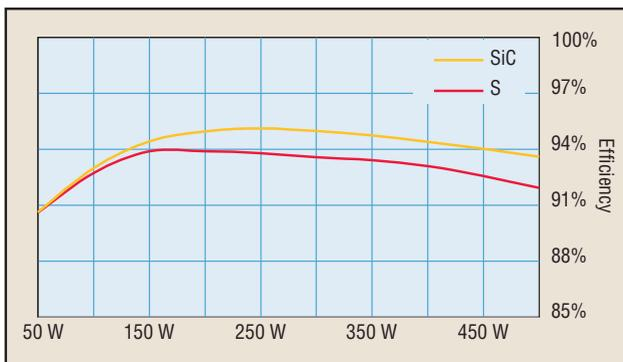
**Fig. 3.** Low-line (90 Vac) efficiency comparisons for an 80-kHz, 500-W PFC front-end converter built with ultrafast Si rectifiers or Cree's
