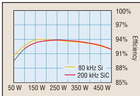
**Fig. 9.** Efficiency of PFC front-end built using low-frequency Si-based design vs. high-frequency SiC-based design.
