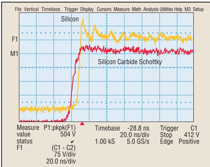
Fig. 6. SiC vs. Si turn-off noise in PFC front-end converter.
