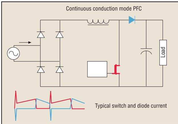
**Fig. 2.** Typical MOSFET and diode current waveforms.
