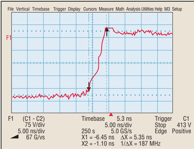
Fig. 5. SiC Schottky turn-off slope in PFC front-end converter.
