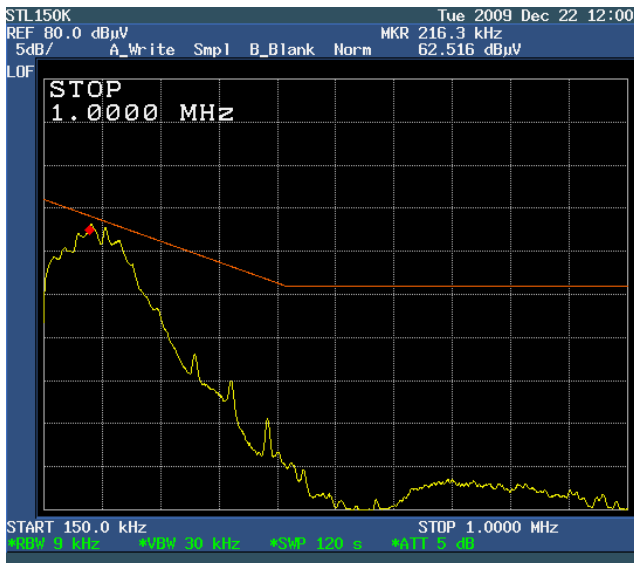
Figure 10: Frequency sweep from 150kHz to 1MHz Vin=208V RMS and Pout=650W
