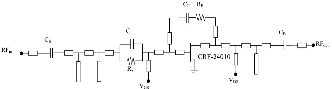
Fig. 3. Schematic diagram of broadband 5 W power amplifier.
