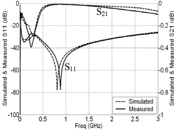
Fig. 2. Simulated and measured S-parameters of broadband choke.
