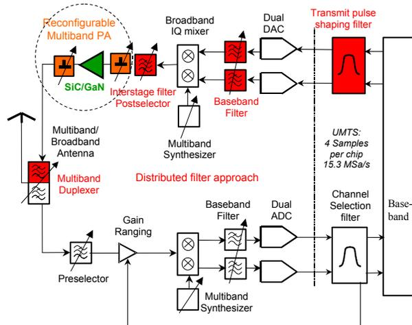
Fig. 12: Architecture of frequency agile basestation system
