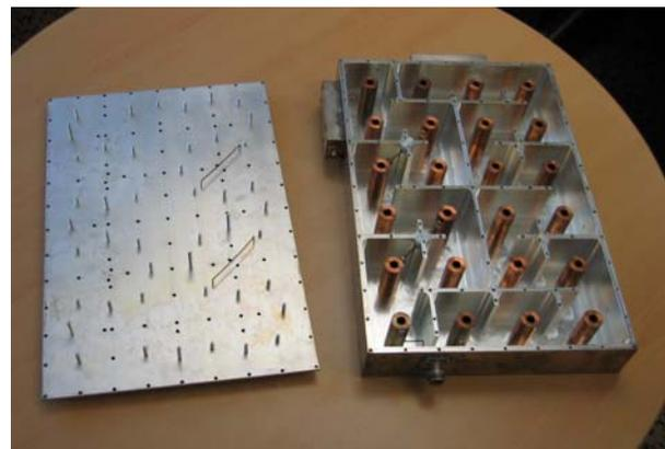
Fig. 3: Typical Duplex-Filter with a UMTS basestation
