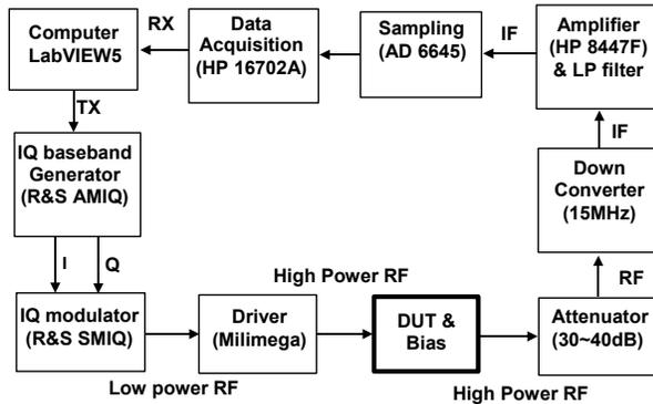
Fig. 9: Test Set-up for analyzing memory effects
