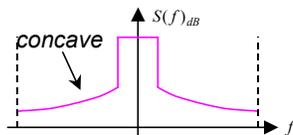
Fig. 4: Principal spectral shaping of a UMTS signal with memory contained non-linear amplification
