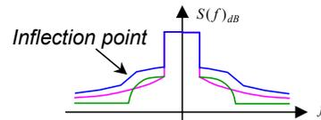
Fig. 5: Principal spectral shaping of a UMTS signal with memory contained non-linear amplification
