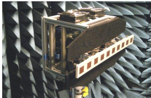
Fig. 1 Linear array of dual polarized antennas on the DAR prototype.
