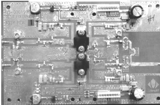
Figure 4. 60W Doherty Amplifier Prototype
