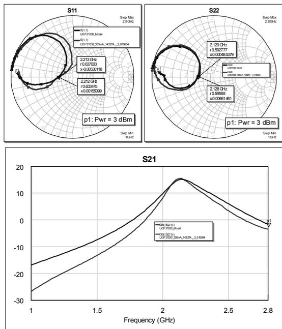
Figure 1. Fits to s-parameter data for UGF21030
