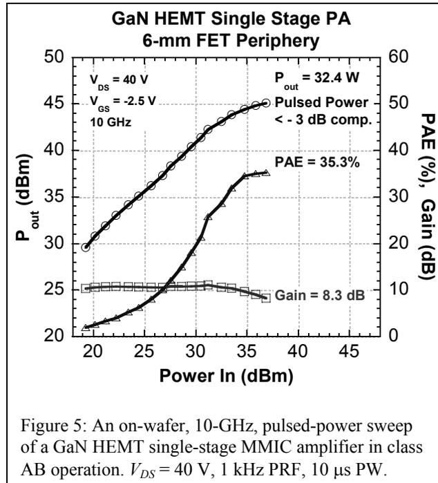
Figure 5: An on-wafer, 10-GHz, pulsed-power sweep of a GaN HEMT single-stage MMIC amplifier in class AB operation.  $V_{DS} = 40 \text{ V}$ , 1 kHz PRF, 10  $\mu\text{s}$  PW.
