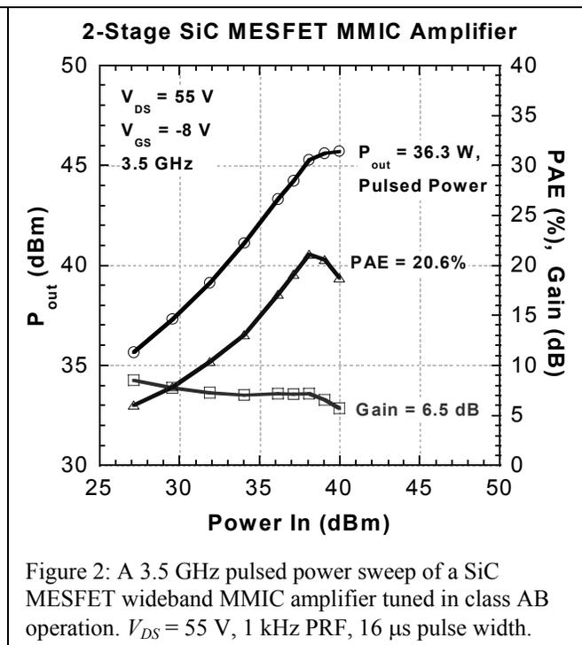
Figure 2: A 3.5 GHz pulsed power sweep of a SiC MESFET wideband MMIC amplifier tuned in class AB operation.  $V_{DS} = 55$  V, 1 kHz PRF, 16  $\mu$ s pulse width.
