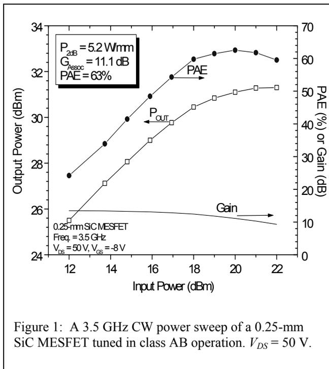
Figure 1: A 3.5 GHz CW power sweep of a 0.25-mm SiC MESFET tuned in class AB operation.  $V_{DS} = 50$  V.
