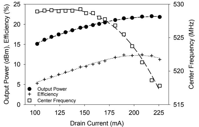
Fig. 4. Change in center frequency and oscillator efficiency as the drain current is varied from  $70$  to  $270\ \text{mA}$ . The drain voltage is held constant at  $6.0\ \text{V}$ .
