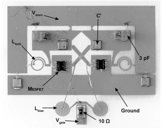
Fig. 3. Photograph of the assembled oscillator circuit.
