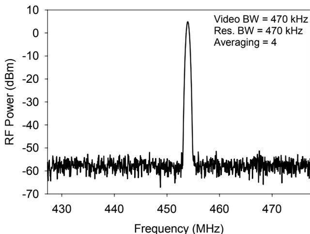
Fig. 9. Spectrum of 453 MHz signal measured at a substrate temperature 475 °C. The drain is biased with 7.85 V and 111 mA. The output power is 4.9 dBm.
