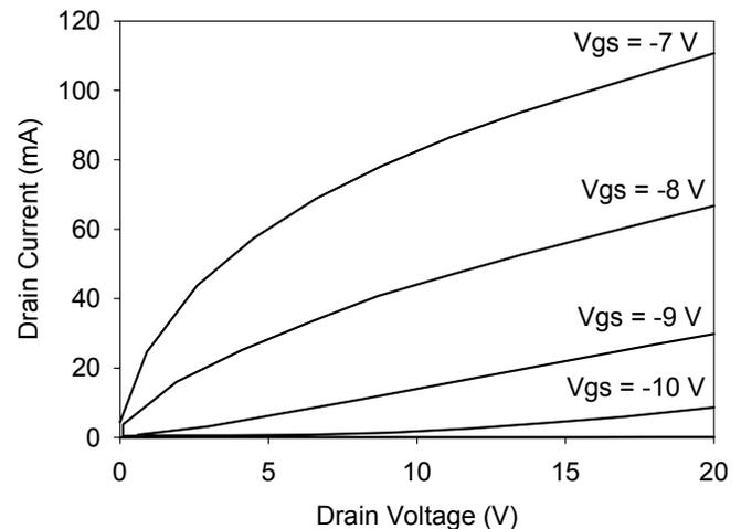
Fig. 1. DC current-voltage relationship of SiC MESFET at gate voltages of -7, -8, -9, and -10 V.
