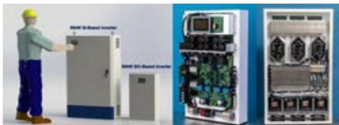
Figure 3: (Left) A relative size comparison of a typical 50kW Si IGBT string inverter and the 50kW SiC-based string inverter demonstration developed by Cree, Inc. (pictured, front and back, on the right)
